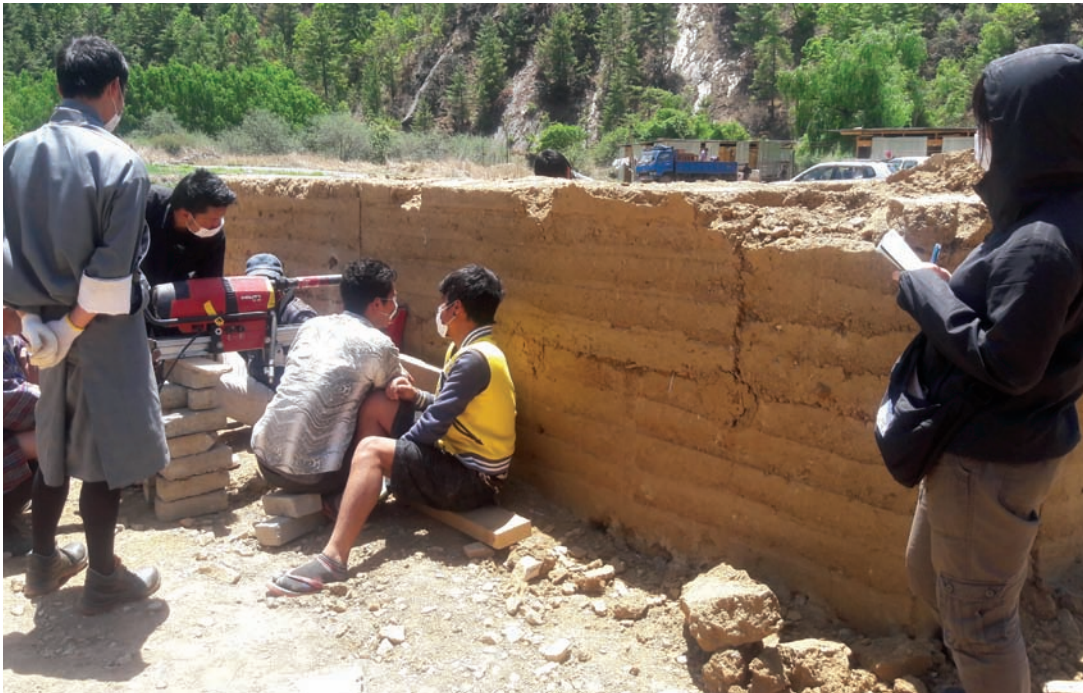
Technicians drill into a mud-rammed wall to draw samples to be used to determine the level of earthquake resistance of traditional buildings
